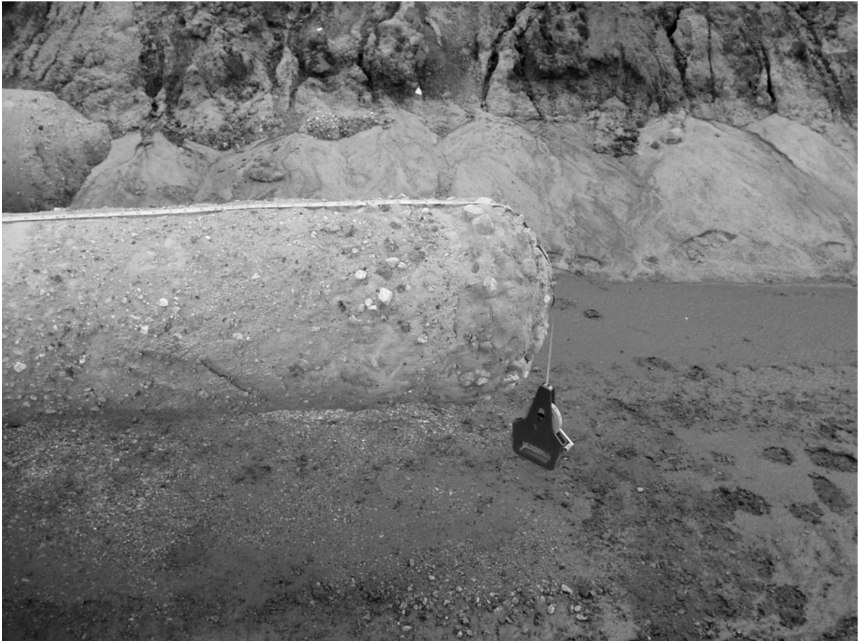
Figure 13. Tip of Pile 42 showing gravel from Layer 5 embedded into the pile.
