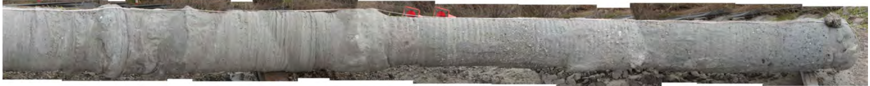
Figure 14. Composite photo of exhumed and cleaned APGD Pile 42.
