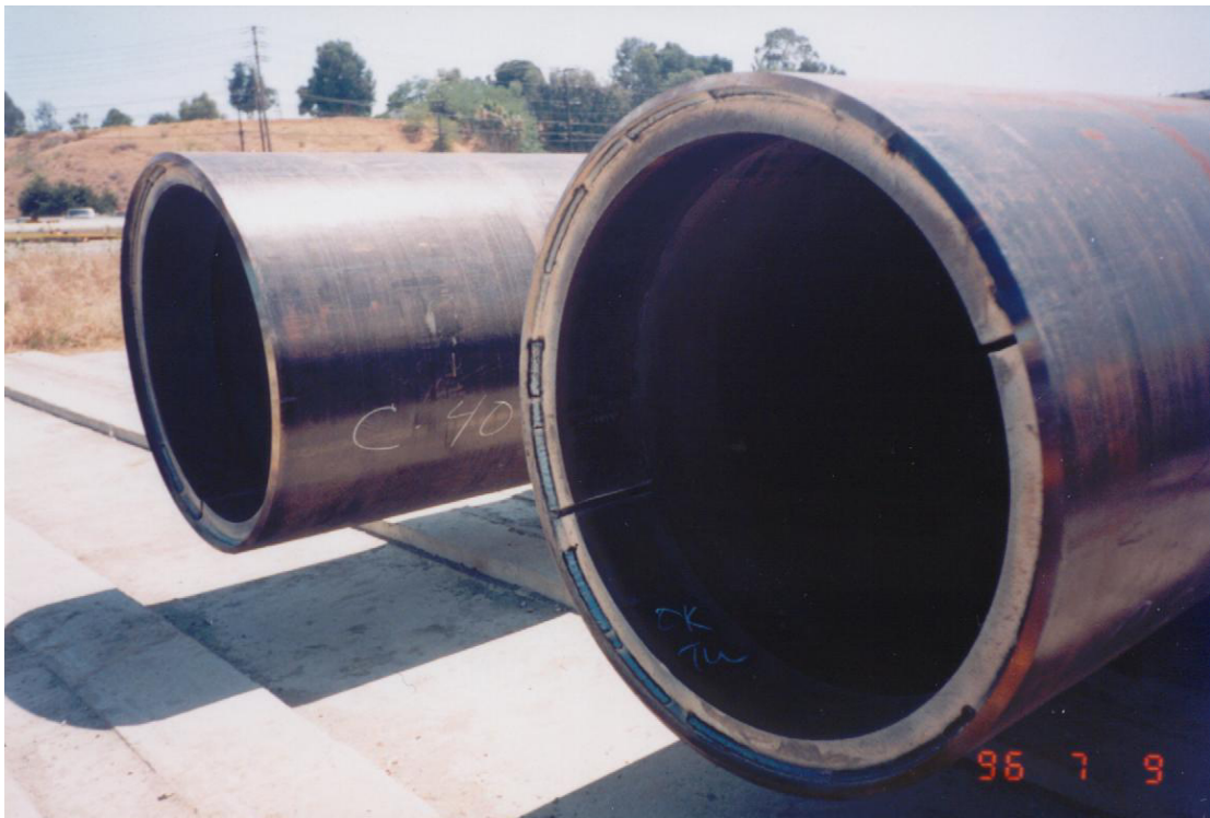
1.37-m (54-inch) Pipe Piles with welded shoes
